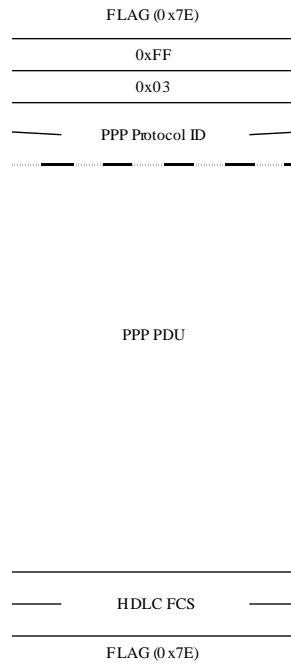
Figure 5-1: HDLC-like-framed PPP PDU
