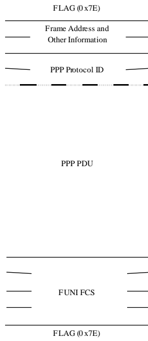
Figure 5-5: FUNI-based, VC-multiplexed PPP PDU
